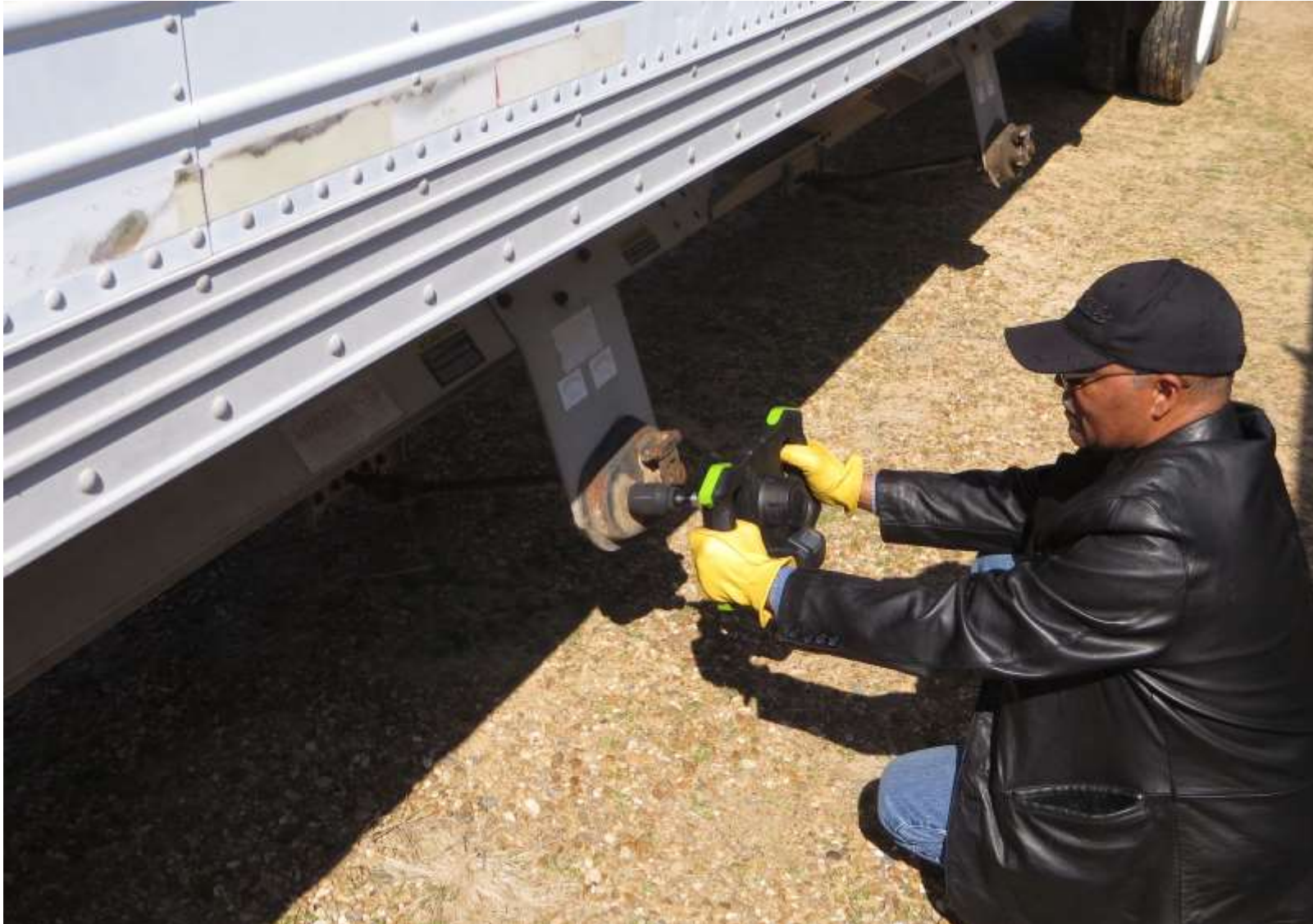
Hopper door opened/closed directly w/o TED, no problem if done correctly
